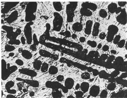
Figure 4 Microstructure of furnace-cooled hypoeutectic alloy containing 50 wt % As_2Te_3 /50% SnTe. Primary crystals of SnTe (black) plus eutectic. Etchant: 1 part CrO_3 : 1 part Eden's reagent ( \times 90 ).
